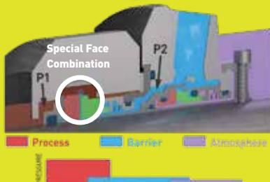
Simple low-cost support system delivers the benefits of a dual pressurized seal, replacing more complex, expensive support systems
